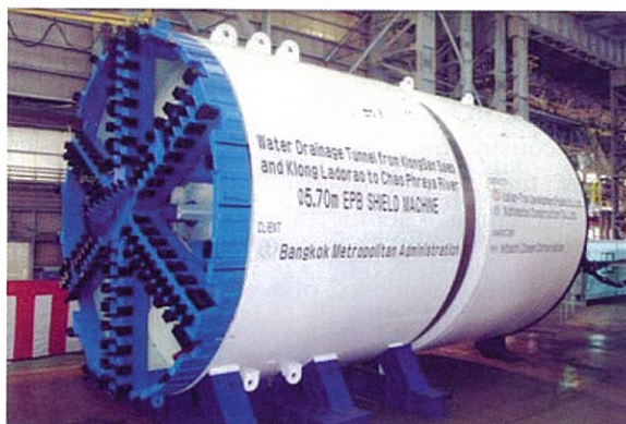
EPB shield, 5.70 m diameter for the Water Drainage Tunnel Project from Sansaeb canal and Ladprao canal to Chao Phraya River
